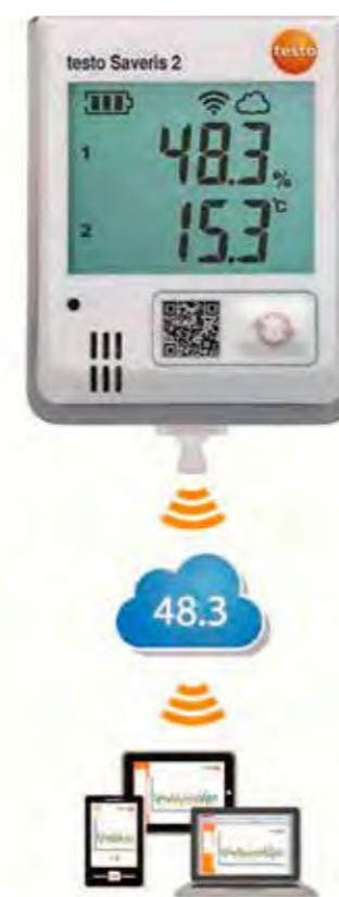
Figura 4. Sensor TESTO SAVERIS II
